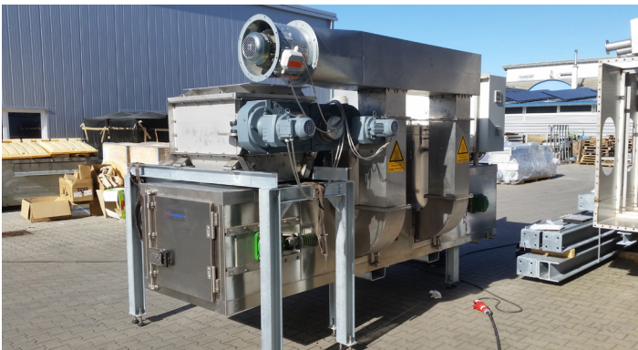
Wet material feed hopper and the roller press above the feed module, exhaust air ducts and exhaust air fan on the right
