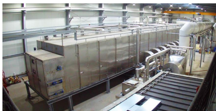
View from the end of Belt Dryer BD 3000/16 with Return module and Exhaust air fan
