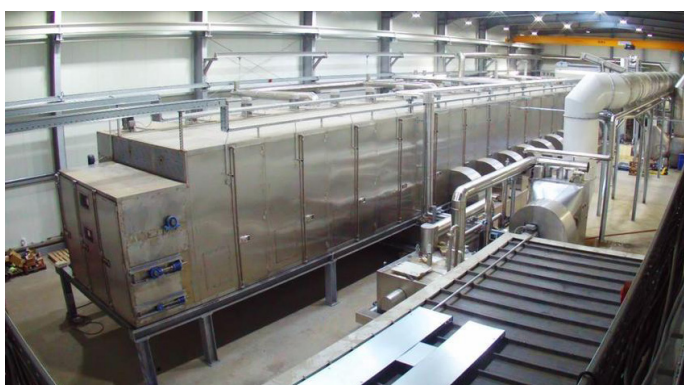
View from the end of Belt Dryer BD 3000/16 with Return module and Exhaust air fan
