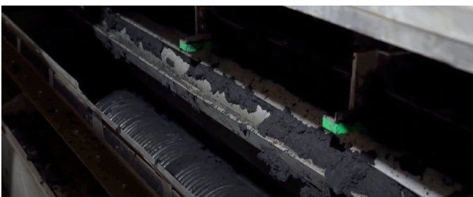
Feed unit with distribution slide and roller press
