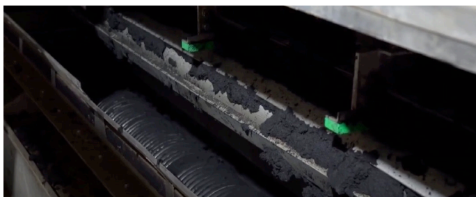
Feed unit with distribution slide and roller press
