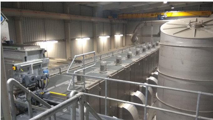
BD 3000/11 belt dryer with distributor/dosing unit and condenser
