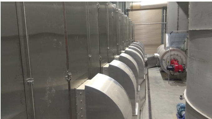
Burner (red) with combustion chamber and subsequent supply air fan for transporting the hot gas into the belt dryer
