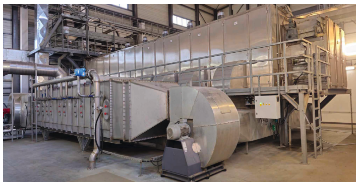
Belt Dryer BD 3000/8 with direct operated horizontal condenser and exhaust air fan
