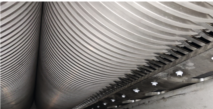
Roller press with scrapers (view from below)
