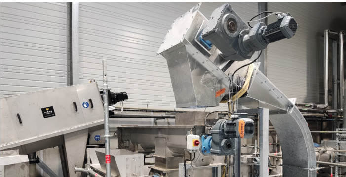
Back-mixing: Trough chain conveyor transports dry sludge into dosing screw
