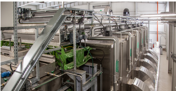
One line of BD 3000/6 belt dryer with feeding unit
