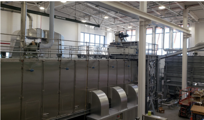
Belt Dryer BD 3000/6 with air duct, inlet unit and wet cake storage hopper
