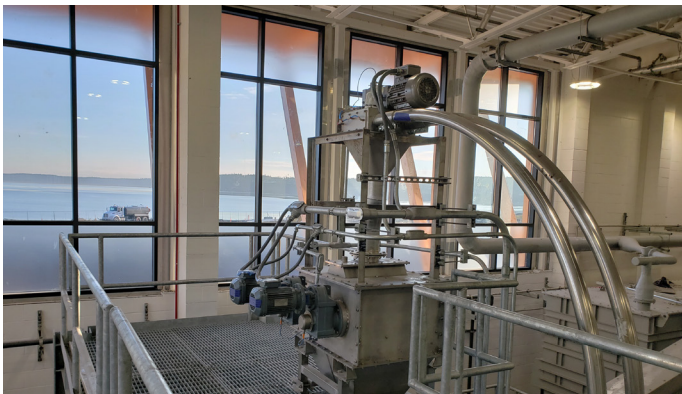
Tubular drag chain conveyor (dry product) to crusher (drum mill)
