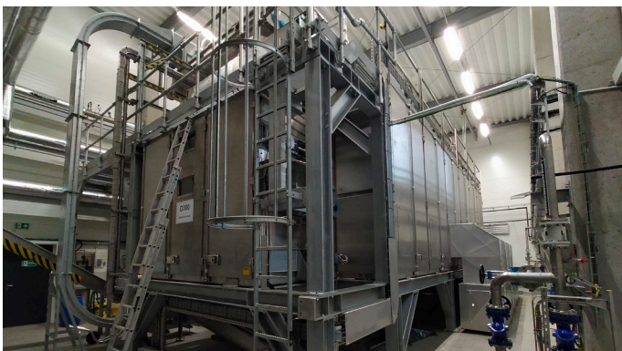
Belt dryer BD 3000/6 with backmixing
