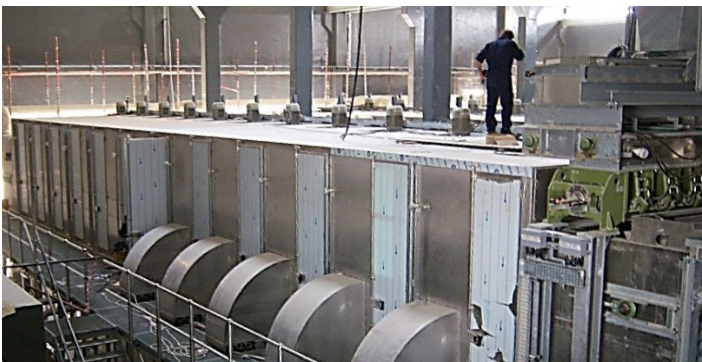
One line of the Belt Dryer BD 3000/12 with dryer inlet unit
