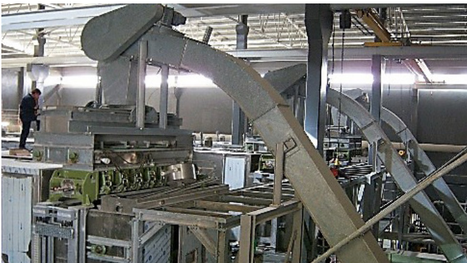
Trough chain conveyor for dewatered sewage sludge to the inlet unit (3x)
