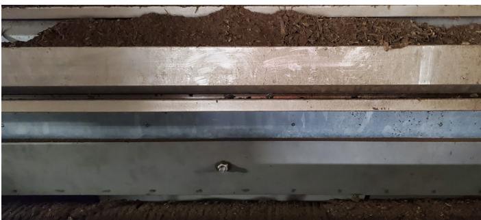
Pre-dried material above roller press for transfer to upper dryer belt
