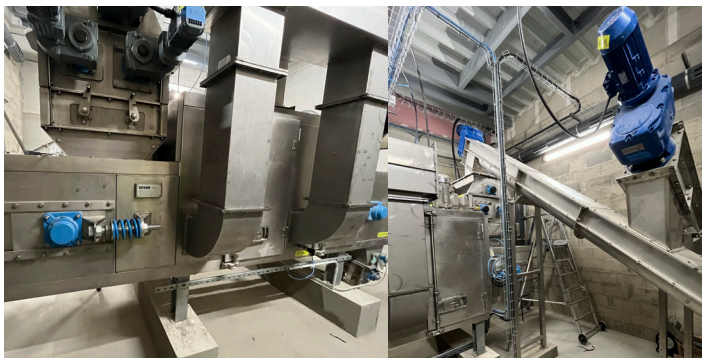
Left: Pilot dryer with feed unit and exhaust air ducts Right: Material feed via screw conveyor
