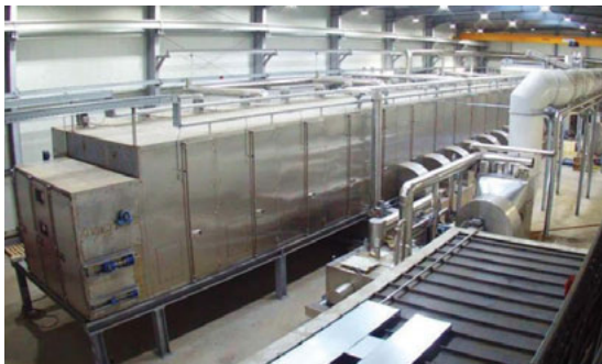
Belt Dryer BD 3000/16 with heat recovery system
